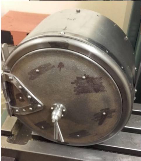
Drilling 44 holes in smokebox and rings
